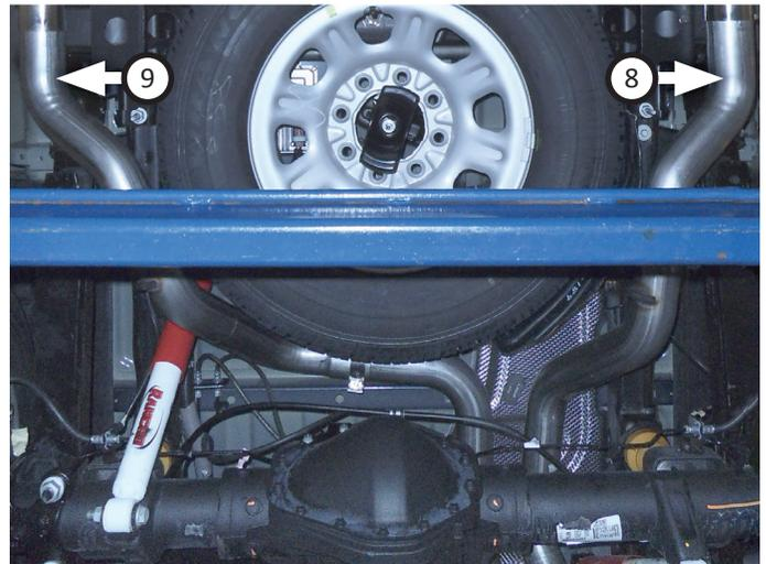
12. Place (x2) **tips (10)** onto exit pipes and tighten inlets. Rotate exit pipes and tips to desired distance from body or bumper, so angle cut on tips are properly positioned.
