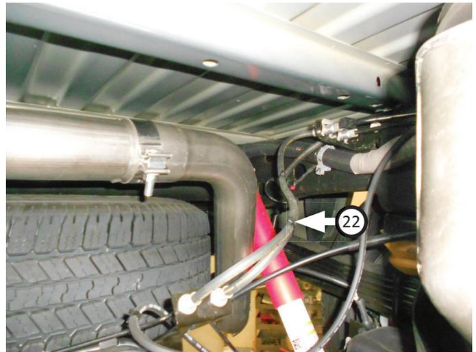
14. Fit (x7)  $\frac{7}{16}$ " (20) and  $\frac{1}{2}$ " (21) hanger keepers onto each sideways hanger.
