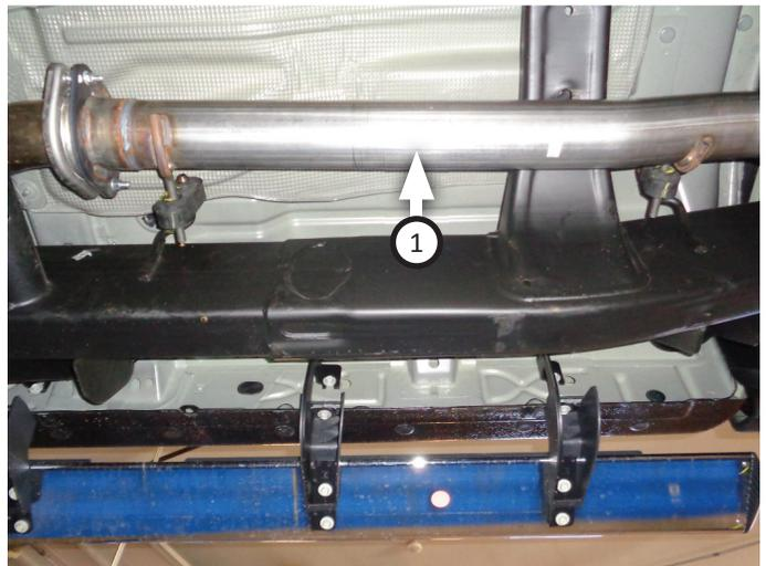
7. Place **clamp (13)** onto **muffler (2)** then connect it to inlet pipe. Tighten clamp just enough to allow for adjustment then place (x2) **clamps (12)** onto muffler outlets.
