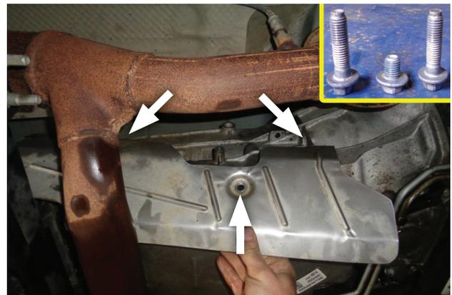
4. Remove bolts (x3) and side cover from passenger side of transmission. Retain for later re-use.
