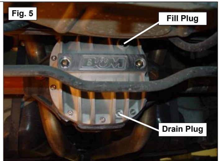
17. Fill with factory recommended gear oil using the B&M Differential Cover fill plug hole. Add gear oil until oil runs out of the **axle housing fill level hole**. (Not the Fill Hole on the cover)
