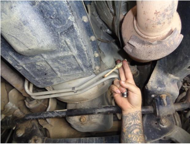
6. Remove the stock dipstick and wipe it off with a clean rag. Then reinsert it, allowing it to seat fully, and remove it again.
