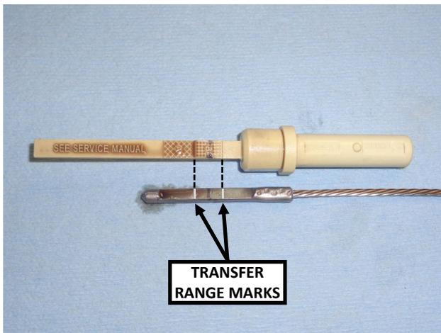
25. Transfer the fluid level range (Max / Min) marks from the stock dipstick to the B&M dipstick. Use a scribe, hacksaw blade or the sharp edge of a needle file to permanently mark the dipstick. Then reinstall the B&M dipstick.
