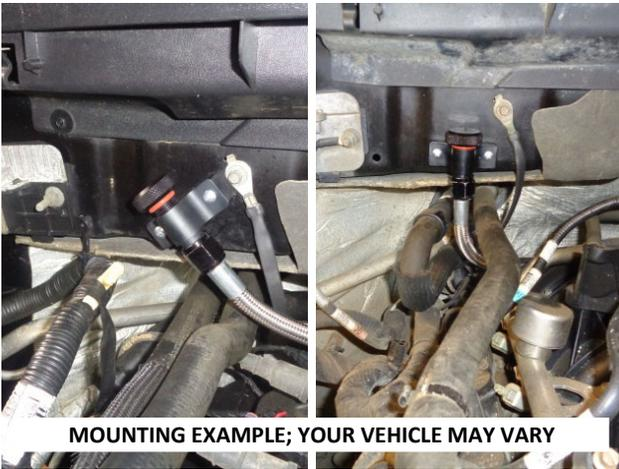
18. Use cable tie(s) to secure the dipstick tube, if required. Fasten the adapter to the chosen location on the firewall using the two self-tapping screws (4).
