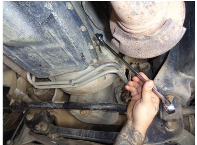
15. Install the dipstick tube fitting (1) in the transmission fill port.
