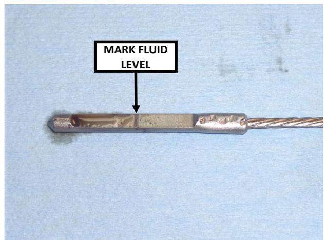
23. Remove B&M dipstick, wipe it off, and reinstall it all the way (knob fully hand tight). Then remove the dipstick again, mark the fluid level with a marker or grease pencil, and turn off the vehicle.
