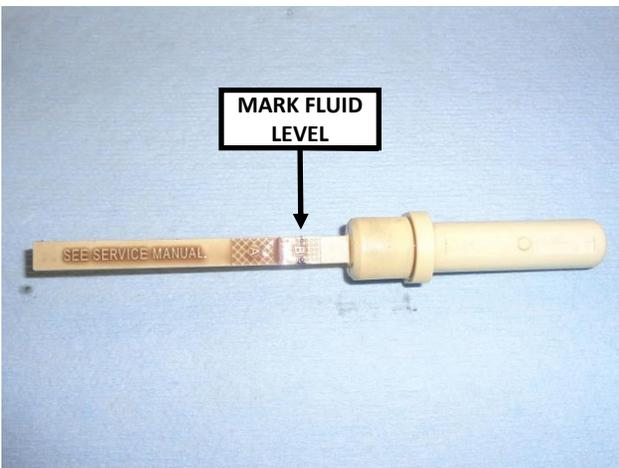
7. Mark the fluid level on the dipstick with a marker or grease pencil and carefully set it aside.
