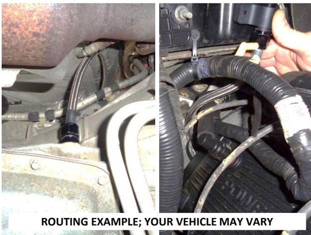
13. Route the tube (2) between the transmission and engine compartment, based on your observations in Steps 9-12.
