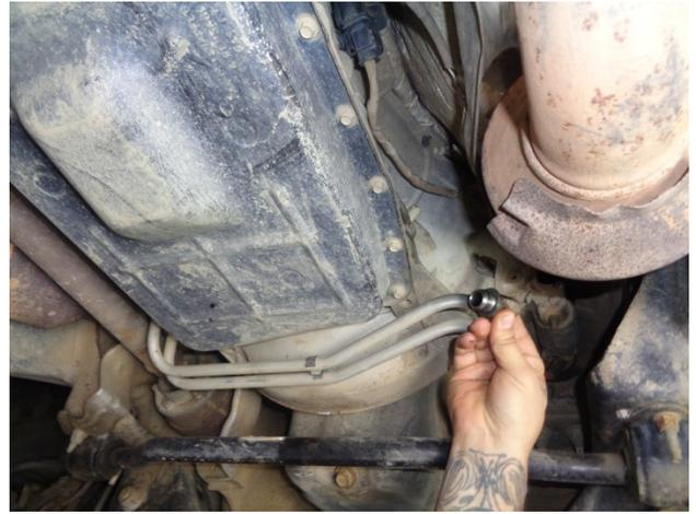
14. Remove the fill cap. If hot (expanded) fluid begins to run out of the port, reinstall the cap, start the vehicle and run it at idle, then remove the cap.
