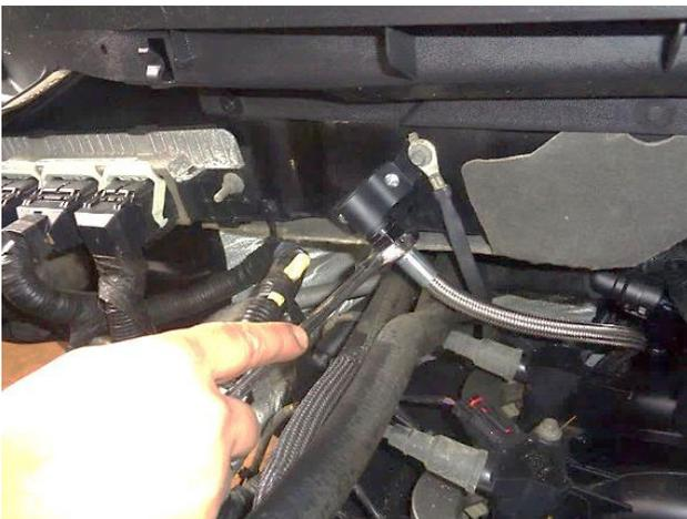
19. Tighten the upper tube nut.
