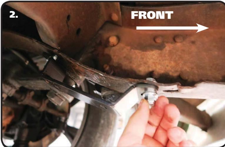
2. The Sway Bar Mount attaches to the frame using the holes from the OEM mount. The end of the frame bracket with the angled bends goes forward. Attach the bracket using a 3/8"-16 x 1 1/4" bolt, 3/8"-16 Nylok nut and a 3/8" Flat Washer on top and bottom. The same hardware setup is used in each hole. Repeat on the other side and tighten hardware.
