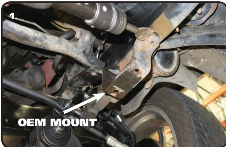
**1.** Some trucks are equipped with sway bar. If your truck has one, the OEM mount will need to be removed to install the StreetGrip Sway Bar. This is done by removing the rivets. The rivets can be removed by chiseling the heads off and driving them out or by drilling the rivets out. The new Frame Mount bolts directly in place of the old mount. If your truck doesn't have a sway bar, the mounting holes will still be in the frame.
