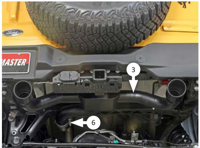
10. Adjust the fit of all exhaust components, maintaining 1/2" clearance and allowing for suspension travel and vibration. Then tighten both clamps. Finally, install the 5 **hanger keepers (12 & 13)** onto each wire hanger.
