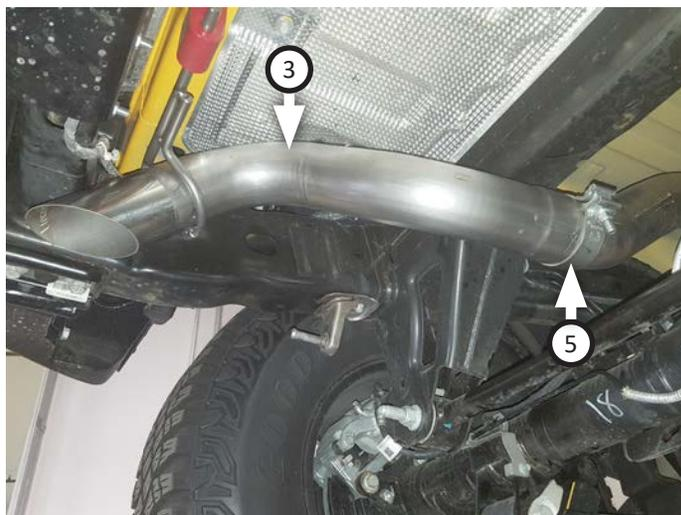
10. Adjust exhaust components for fit; maintaining ½" clearance and compensating for suspension, travel and vibration then tighten all clamps. Finally, fit (x3) **hanger keeper (11,12)** onto each sideways hanger.
