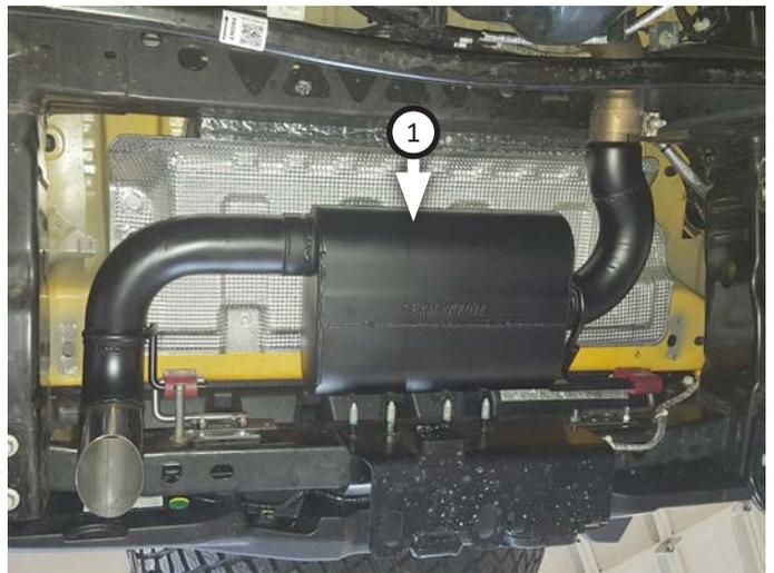
7. Fit (x4) **hanger keepers (9)** onto each hanger.
