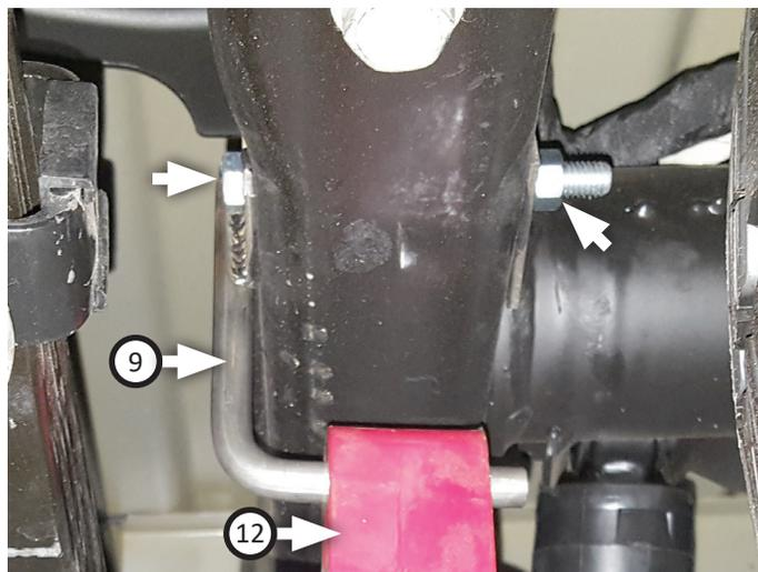
10. Route **left front (3)** and **right tailpipes (4)** over axle then connect them to muffler. Insert their wire hangers into isolators then tighten clamps just enough to allow for adjustment.
