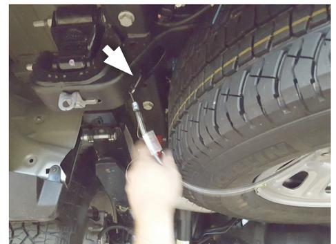
9. Fasten **left frame hanger (9)** to vehicle using **bolt (15)**, **backing plate (13)**, **flat washer (16)**, **lock washer (17)** and **nut (18)** as shown. Then hang **rubber hanger (12)** on frame hanger end.
