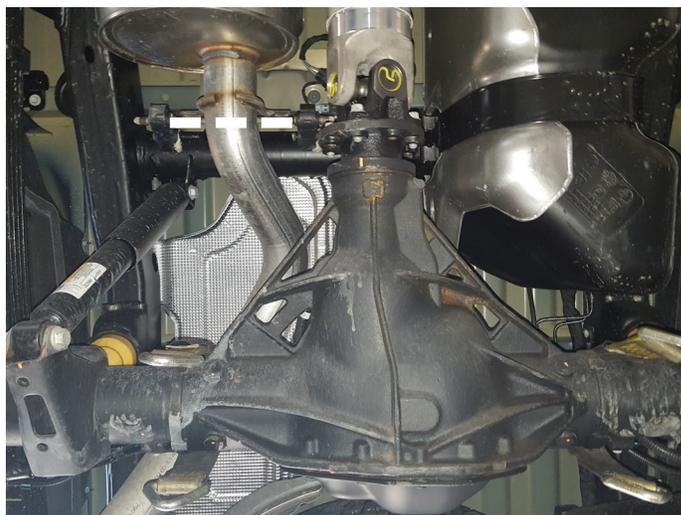
4. Remove nuts (x2) at factory flanged connection behind catalytic converter, separate hangers from isolators on exhaust then remove muffler section. Remove studs (x2) from catalytic converter flange.
