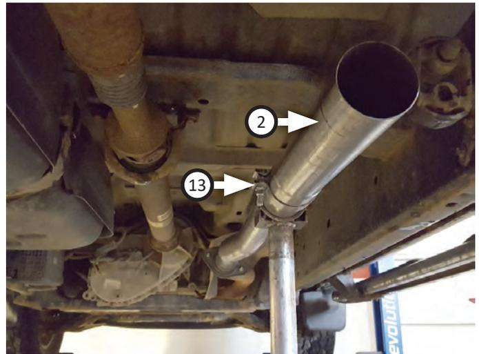
10. Place **clamp (13)** onto **muffler (3)** then connect it to inlet/extension pipe. Tighten clamp just enough to allow for adjustment then place (x2) **clamps (13)** onto muffler outlets.
