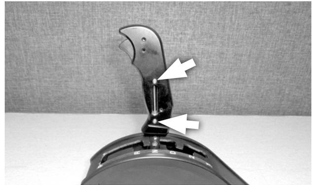
3. Loosen the 2 grip set screws 2-3 turns, then remove the pistol grip assembly from the shift lever.
