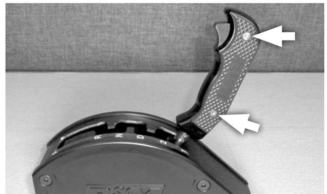
**16. Reinstall the left side grip plate (2 screws).**
