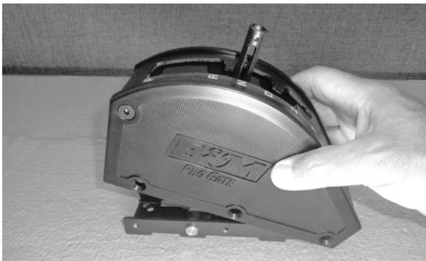
**12. Ensure there is no debris in the shifter mechanism.** Then reinstall the gate plate and cover assembly on the shifter base while guiding the shift lever up through the NEUTRAL position. Secure the cover to the shifter base with 3 screws on each side.
