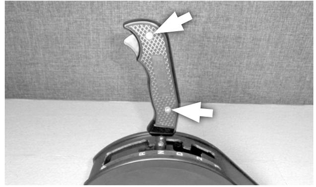
2. Move the shift lever to the **NEUTRAL** position on the right side (away from the PRNDL label). Then remove the left side grip plate (2 screws).
