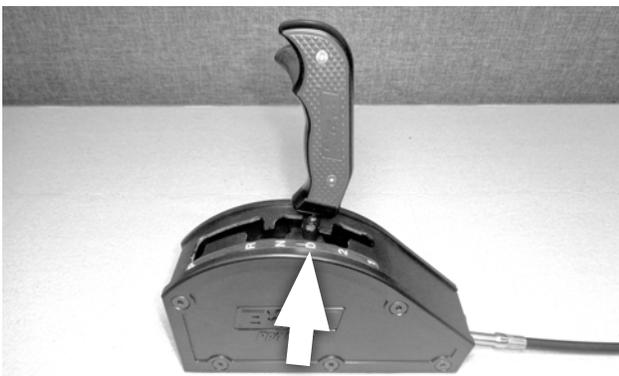
22. **At the transmission, manually move the selector lever** to the DRIVE detent (that is, 3 clicks forward from fully-rearward, or PARK). Then **in the vehicle, move the shifter handle** to DRIVE.
