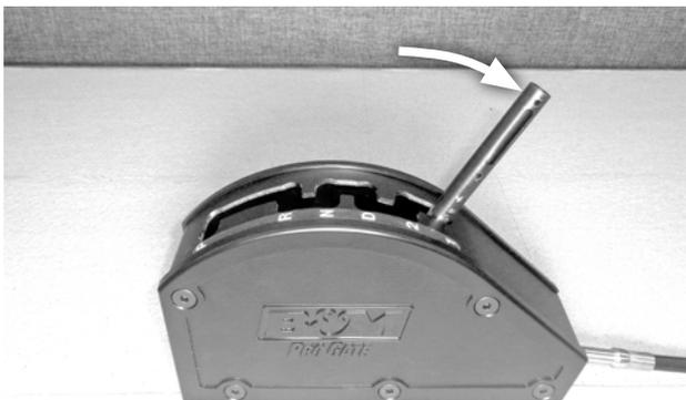
**13. Move the shift lever to LOW (1),** which will allow the lockout plunger on the pistol grip to align more easily with its guide hole inside the lever.
