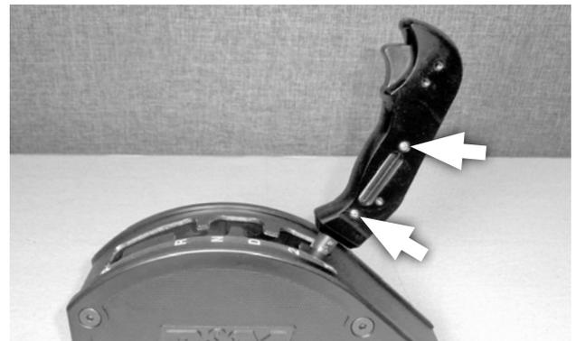
**15. Tighten the pistol grip set screws in an alternating manner** until they are flush with the grip. Test the trigger to verify that it actuates and resets smoothly.
