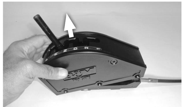
3. Remove the gate plate and cover assembly (3 bottom screws on each side).
