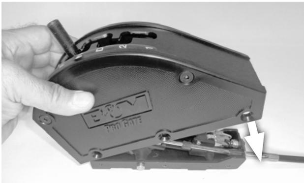
14. Ensure there is no debris in the shifter mechanism. Then reinstall the gate plate and cover assembly on the shifter (6 screws, 3 on each side) according to your shifter's instructions.
