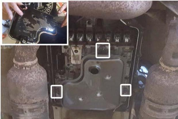
6. Remove (3) bolts then pull transmission pan filter down and off of vehicle.
