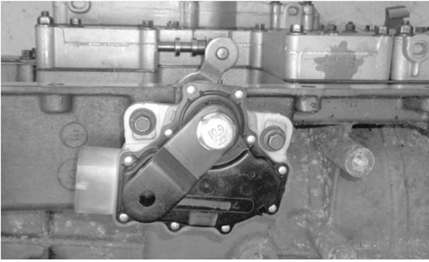
14. Install the selector lever on the shaft, using the supplied M10-1.5 x 20 bolt and M10 washer.
