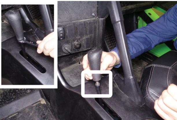
2. Turn off vehicle and chock tires, then carefully remove stock shifter handle.
