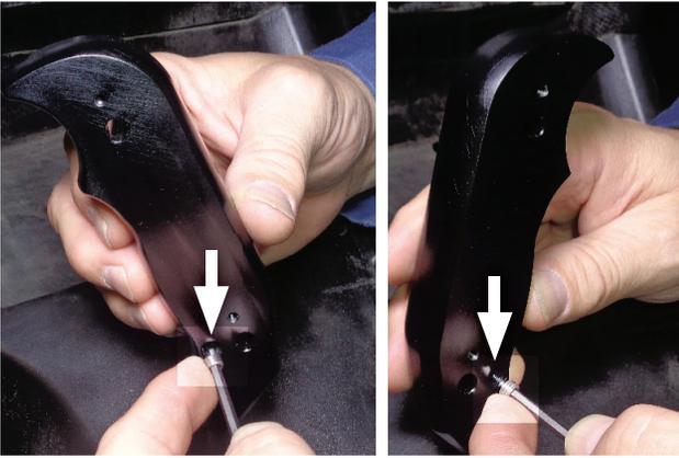
6. Install set screws onto handle body as shown.
