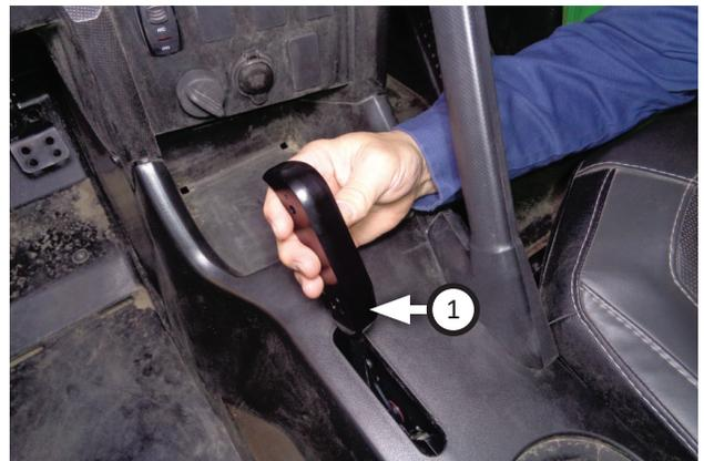
4. Thread **handle body (1)** onto shifter stem. Tighten it fully until it faces dashboard.
