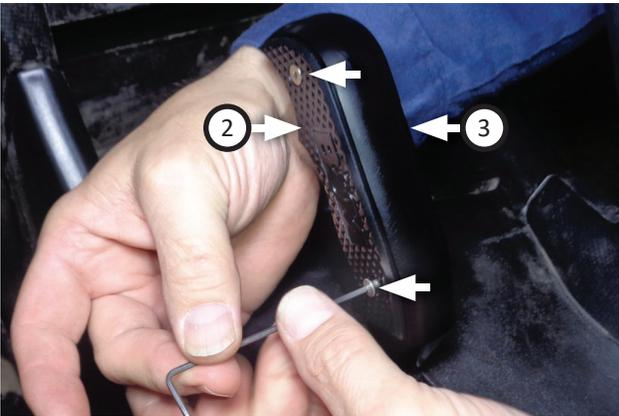
7. Install left (2) and right (3) shifter plates onto handle body using (x4) screws (5).
