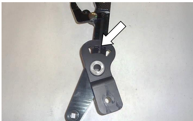
15. Place the shifter gate (4) over the pivot sleeve, so that the selector pin is located in the gate's REVERSE-NEUTRAL (widest) notch.
