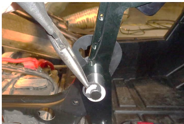
17. Install the retaining clip on the end of the shaft.
