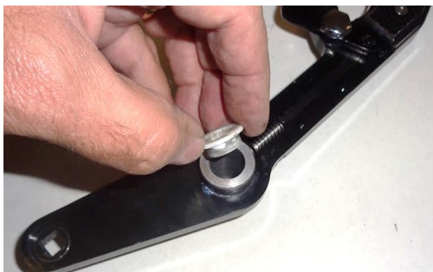
14. Install one nylon bushing in each end of the pivot sleeve in the shift lever assembly (1).
