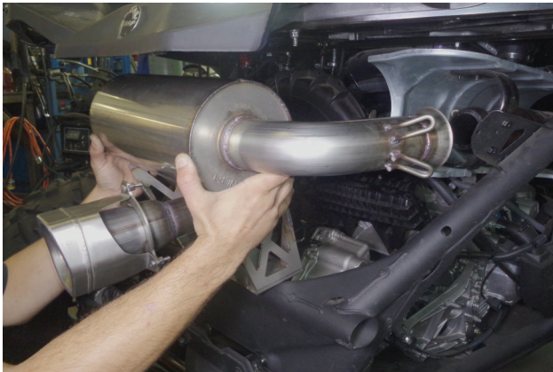
13. Place muffler into place on vehicle.
