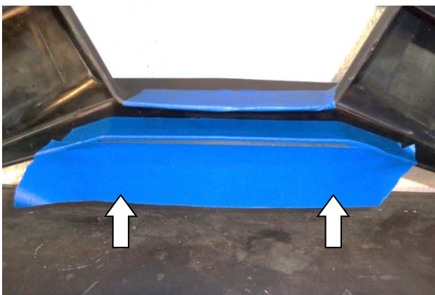
26. Temporarily apply a piece of 2" masking tape parallel to the very bottom edge of the opening, as shown.
